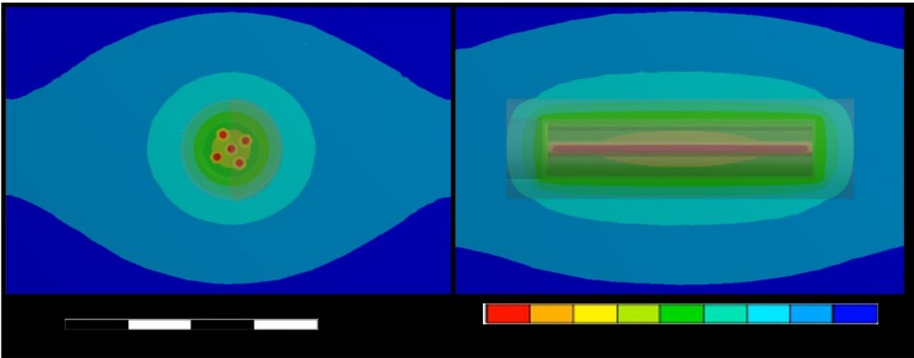
Figure 8. The maximum value of temperature history at the center and surface of the disposal cask and surface of the surrounding bentonite layer.
