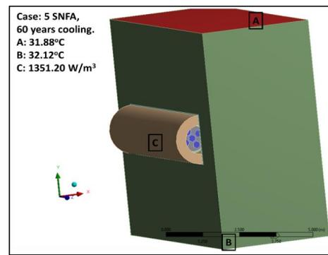
Figure 6. Schematic representation of thermal elements defined in ANSYS Mechanical APDL.
