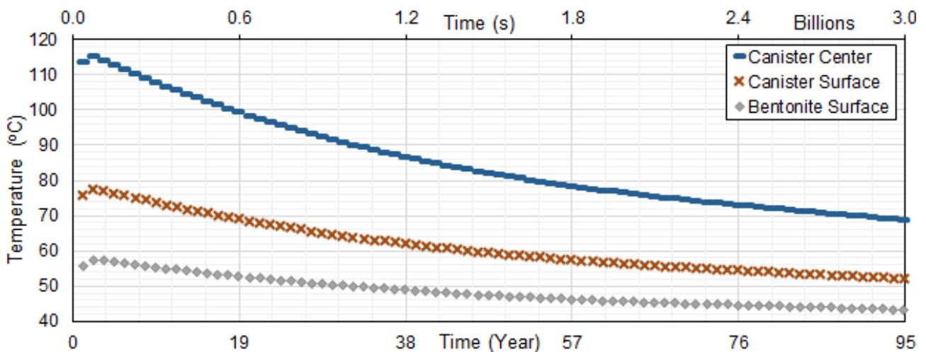
Figure 7. All-time – high temperature distribution of disposal cask and surrounding host rock.
