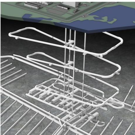
Figure 3. KBS-3H repository concept schematic.
