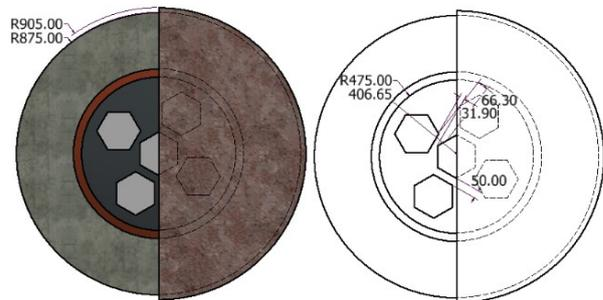
Figure 4. Orientation of VVER-1200 SNFA's in disposal.
