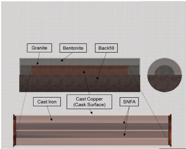
Figure 5. Geometric representation of disposal cask model that used in thermal modeling.
