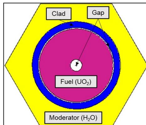
Figure 1. XY cross-section representation of the MCNP input model for the unit cell.
