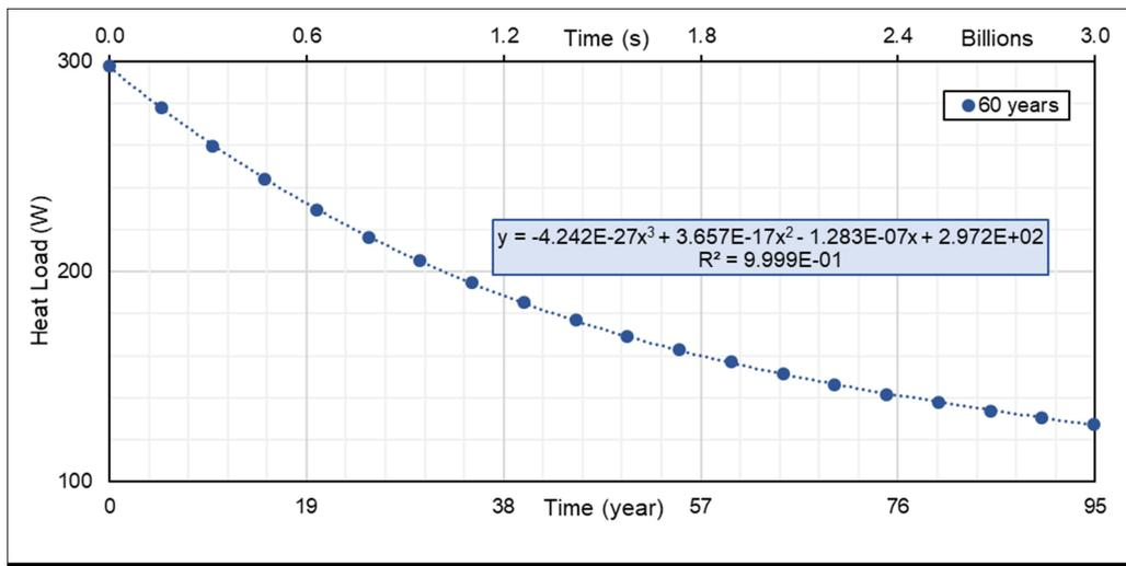
Figure 2. Time-dependent heat load data for a single VVER-1200 SNFA.
