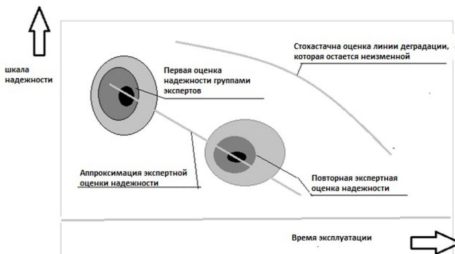
Figure 3. Explanation of expert groups action strategy to determine reliability resources of the equipment by the application of double inspection.
