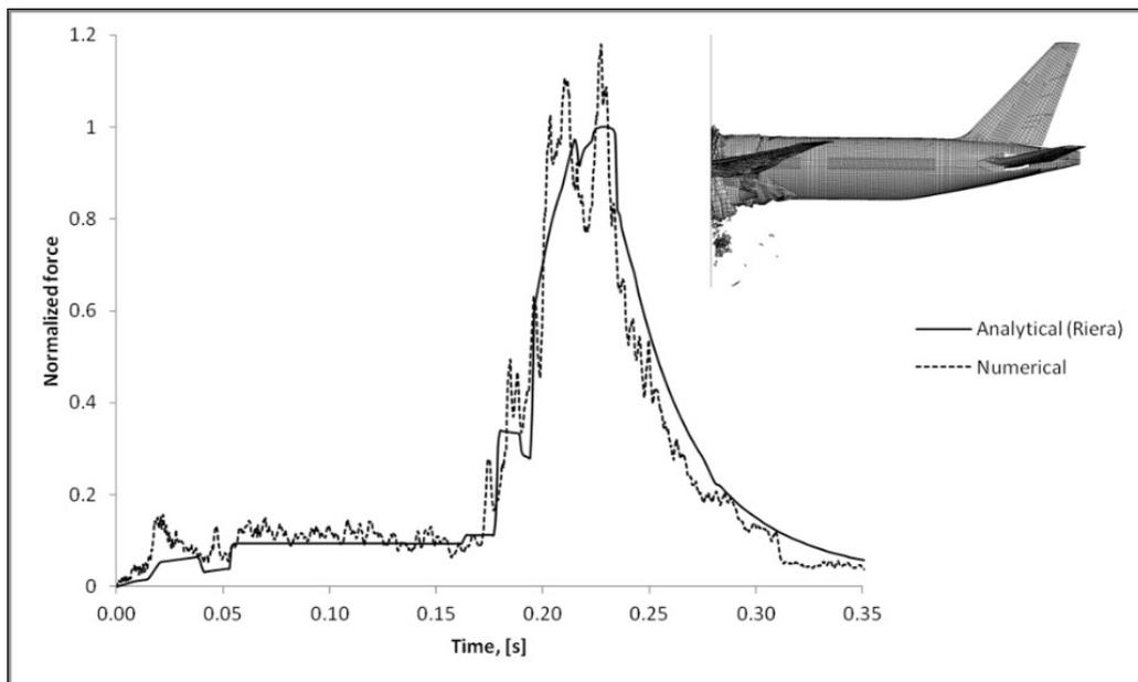
Figure 4. Comparison of analytical and numerical load functions.
