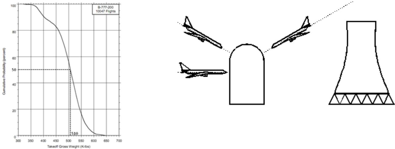
Figure 2. Cumulative probability for takeoff gross weight [3] (left), illustration of possible impact angles (right).
