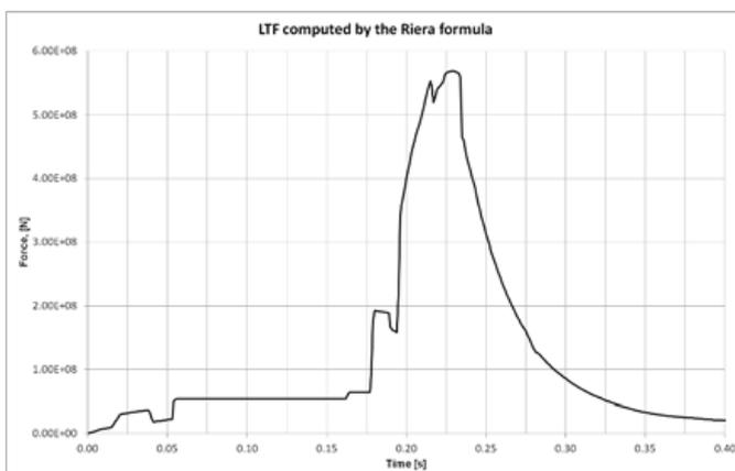
Figure 3. Load function computed by the Riera formula (left) and illustration of the MTI (right).
