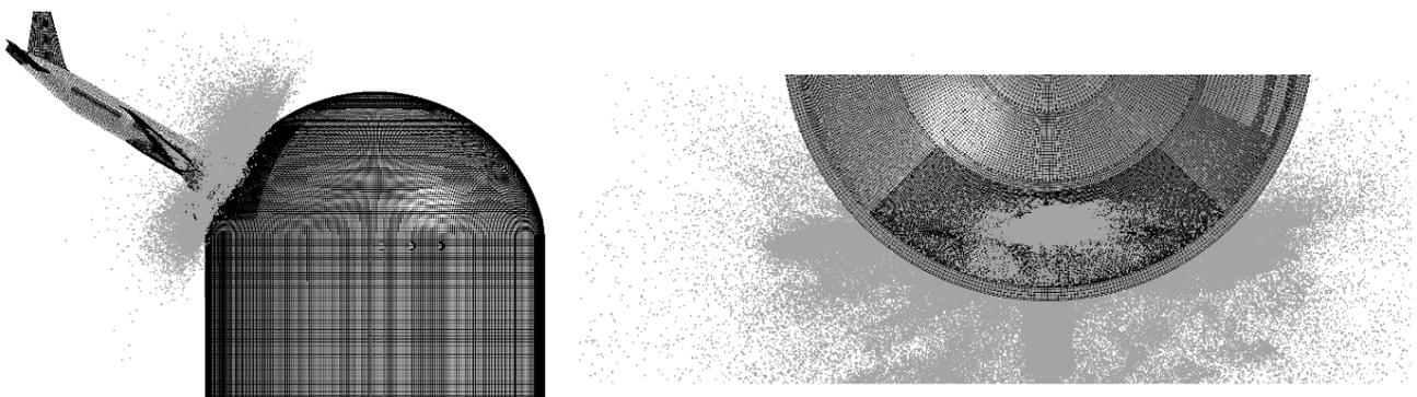
Figure 5. Impact of airliner with SPH model of fuel and payload (left) and SPH particles penetrating through the perforation (right).
