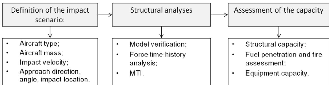
Figure 1. Flowchart for the process of assessment of a NPP due to impact from large airliner.
