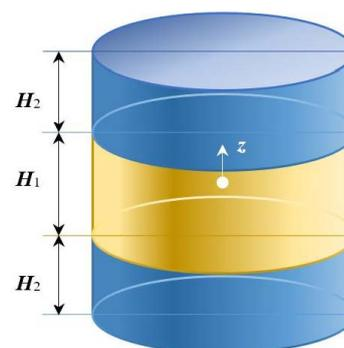
Figure 1. Model of a two-zone flat reactor with symmetry about the center of core.
