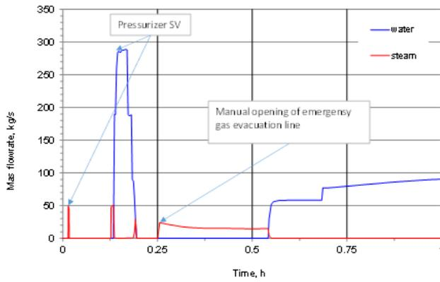
Figure 1. Water and steam mass flow to the containment.
