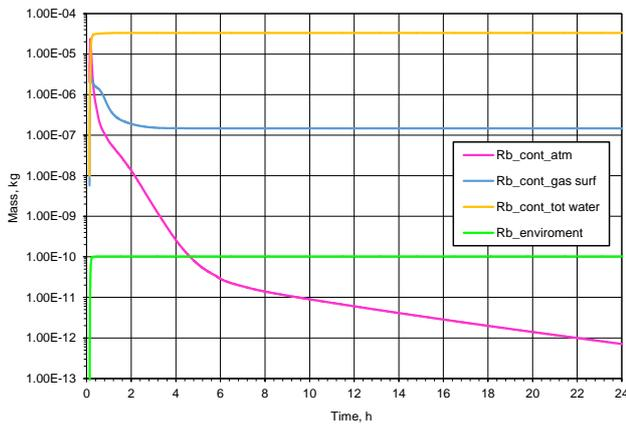
Figure 6. Distribution of Rb in the containment and release into the environment for the period of 24 hours.
