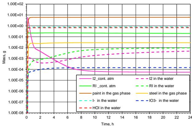
Figure 8. Mass of iodine compounds in the containment atmosphere, on the containment surfaces and in the water.
