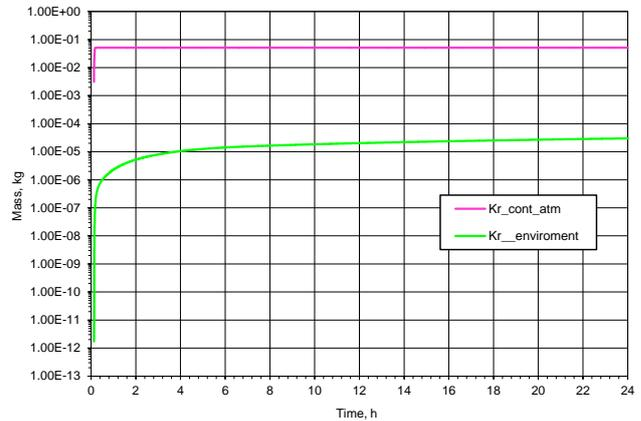
Figure 5. Distribution of Kr in the containment and release into the environment for the period of 24 hours.
