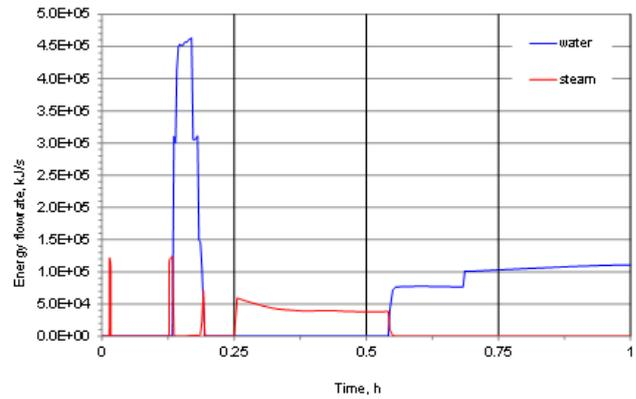
Figure 2. Water and steam energy flow to the containment.
