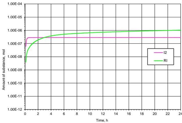
Figure 7. Amount of substance in iodine compounds, released into the environment.
