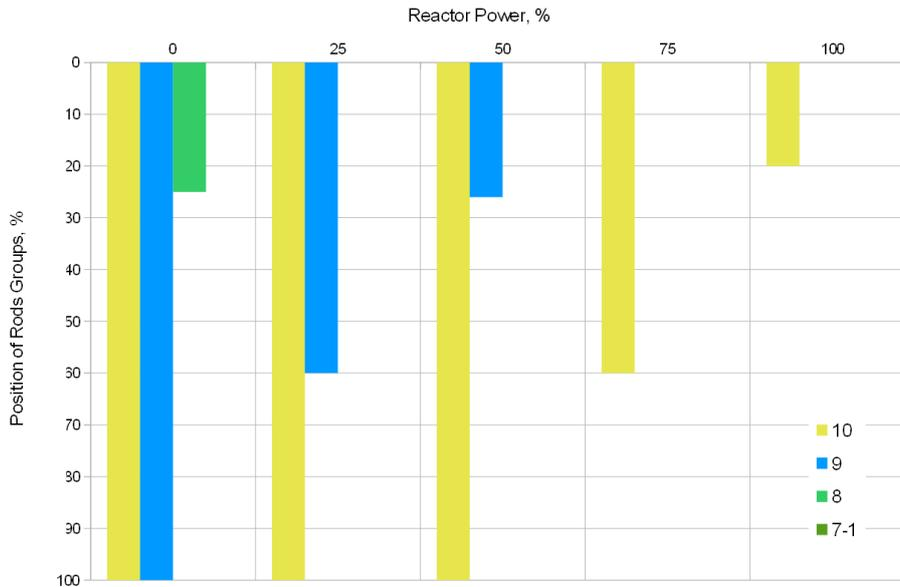
Figure 2. Positions of control rods groups at definite reactor power [1].
