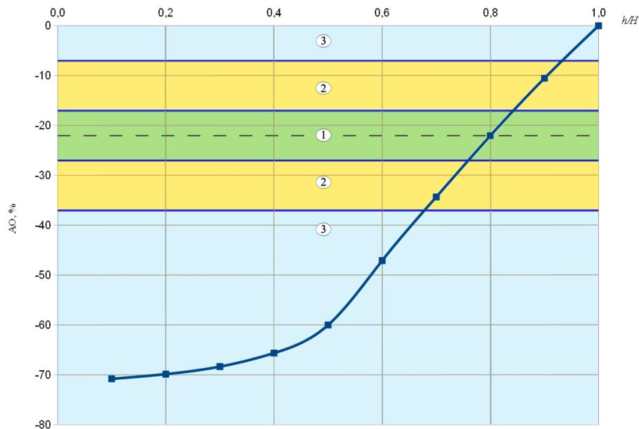
Figure 7. AO depending on the control rods withdrawal. Range of AO: recommended (1); allowable (2); unallowable (3).
