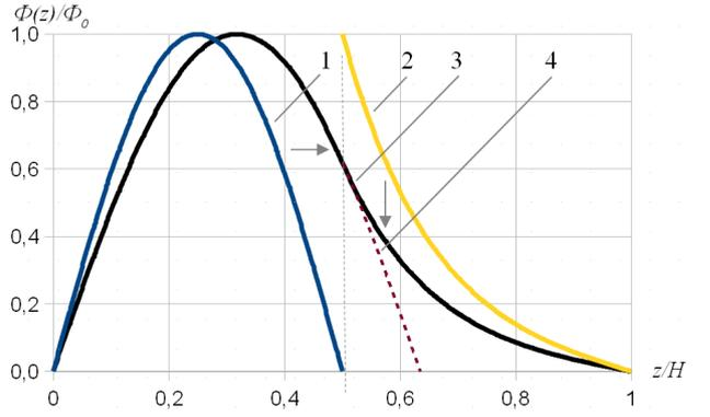
Figure 4. Axial profile of the neutron flux at criticality ( $h = 0.5H$ ):  $Z_1(z) = A_1 \sin(B_{1z}z)$  (1);  $Z_2(z) = A_2 \sinh(B_{2z}[H-z])$  (2); joint solution (3); extrapolation (4).
