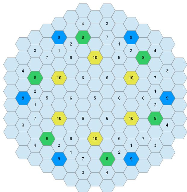
Figure 1. Groups of control rods in core of VVER 1000.
