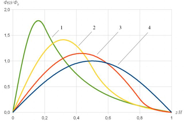
Figure 6. Changing the amplitude and shape of the axial profile of neutron flux depending on the control rods withdrawal  $h/H$ : 0.2 (1); 0.5 (2); 0.8 (3); 1.0 (4).
