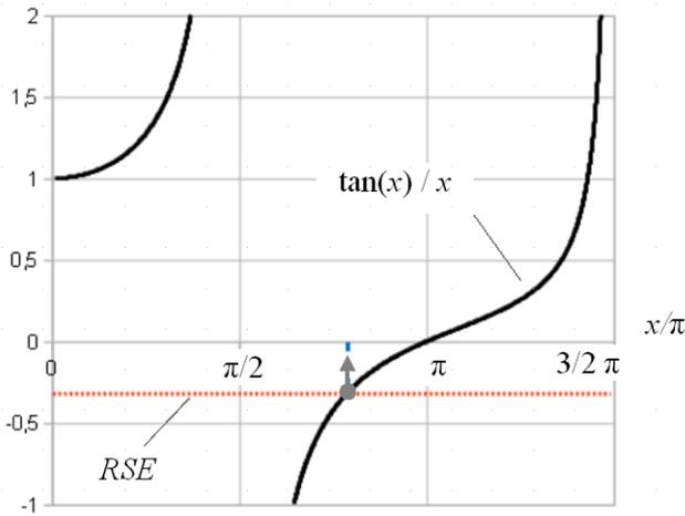
Figure 3. Solution of the criticality equation (at  $h = H/2$ ,  $x = 0.7881\pi$ ).
