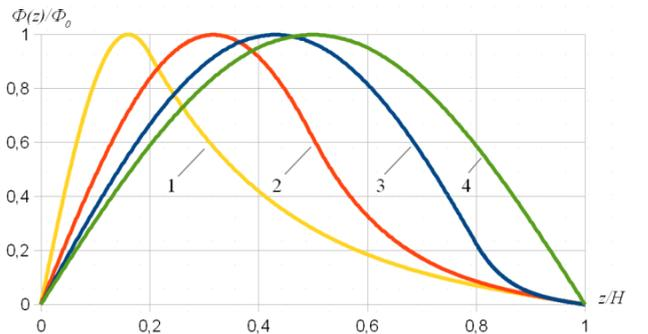
Figure 5. Axial profile of neutron flux depending on the control rods withdrawal  $h/H$ : 0.2 (1); 0.5 (2); 0.8 (3); 1.0 (4).
