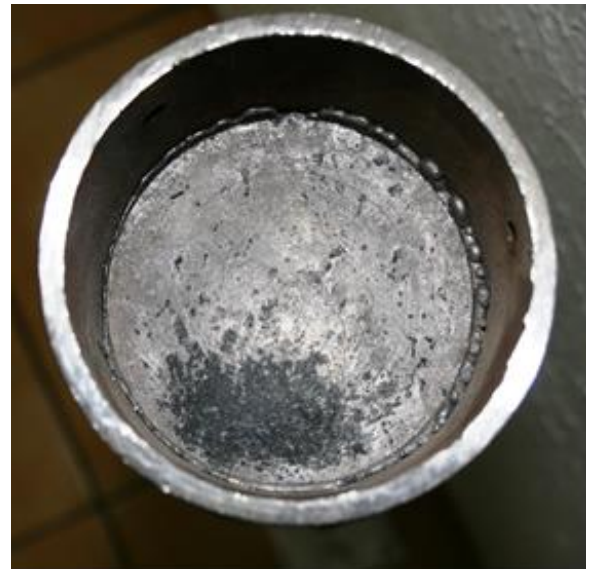
Figure 11. Picture of the frozen melt in the clearance between the plug and the shielding tube.
