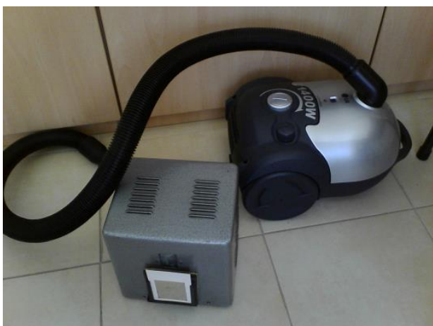
Figure 6. Laboratory set-up of practice “Radioactivity. Determining volume activity of \beta -radioactive aerosols”.
