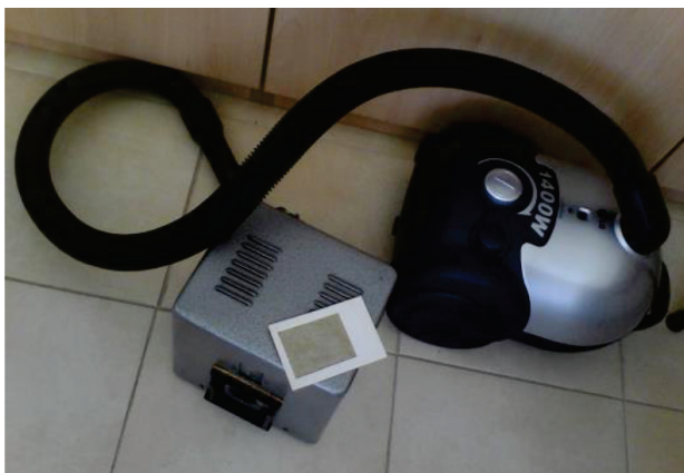
Figure 5. Necessary equipment and materials: aspirator device, framework with air filter.
