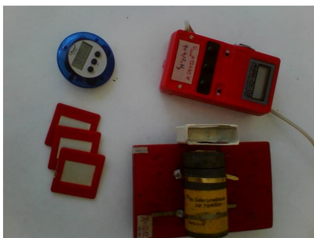
Figure 1. Necessary equipment and materials: lead container with \gamma -source, framework with lamellae of substance under investigation, dosimeter – radiometer and stopwatch.
