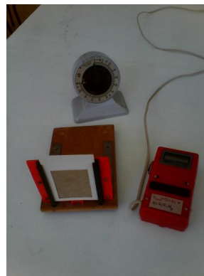
Figure 7. Necessary equipment and materials: mobile rack frame dosimeter – radiometer and stopwatch.
