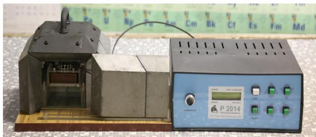
Figure 3. Laboratory radiometric equipment R2014.
