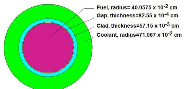
Figure 1. Geometry of PWR pin cell.
