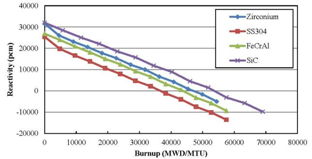
Figure 3. The variation of reactivity with burnup for proposed fuel designs.
