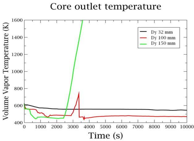
Figure 5. Total blackout and LOCA Dy 32, Dy 100 and Dy 150, one TQ3 pump in operation.
