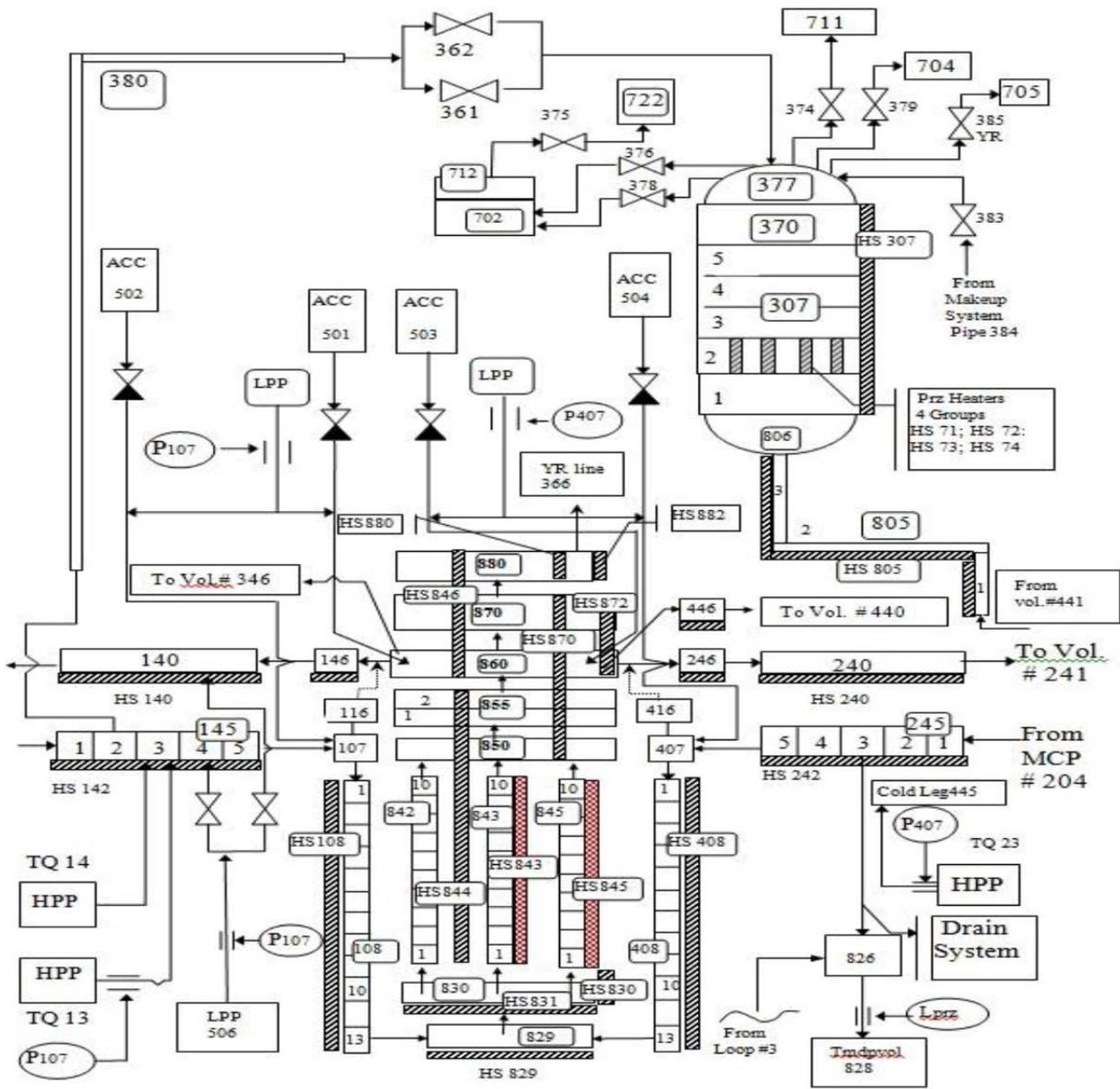
Figure 1. Reactor and Pressurizer RELAP5/Mod 3.3 Four Loops Model.
