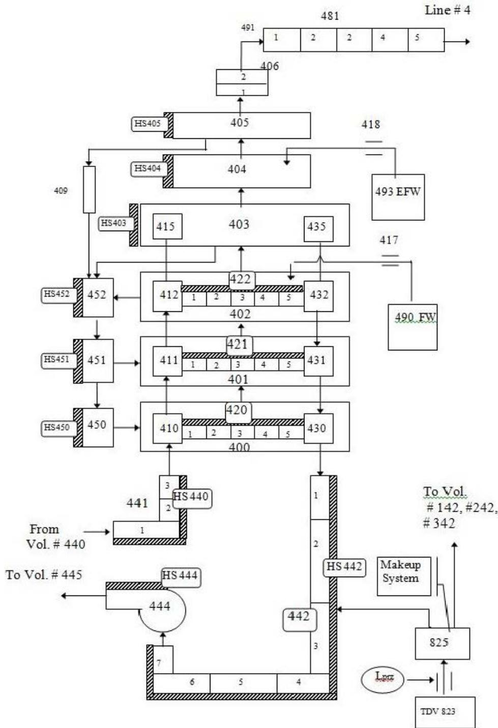
Figure 2. Steam Generator RELAP5/Mod 3.3 Four Loops Model.
