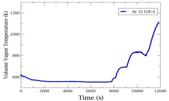
Figure 3. Total blackout and LOCA Dy 32, all 3 TQ4 pumps in operation.
