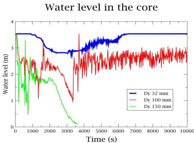
Figure 6. Total blackout and LOCA Dy 32, Dy 100 and Dy 150, one TQ3 pump in operation.
