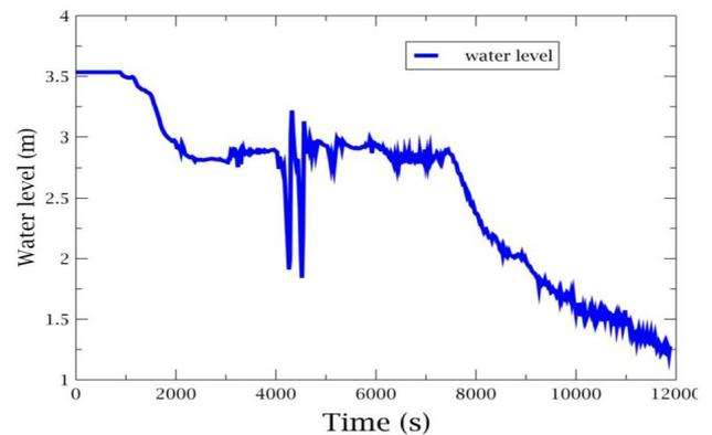
Figure 4. Total blackout and LOCA Dy 32, all 3 TQ4 pumps in operation.
