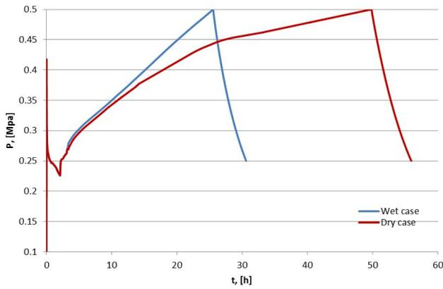
Figure 2. Containment pressure considering dry and wet cavity.
