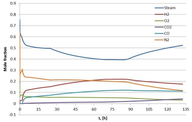
Figure 8. Concentration of the containment atmosphere components – one cavity case.
