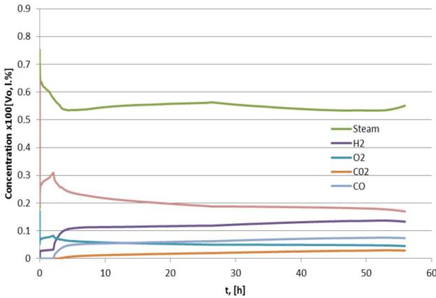
Figure 4. Volumetric concentration of the containment atmosphere components – dry case.
