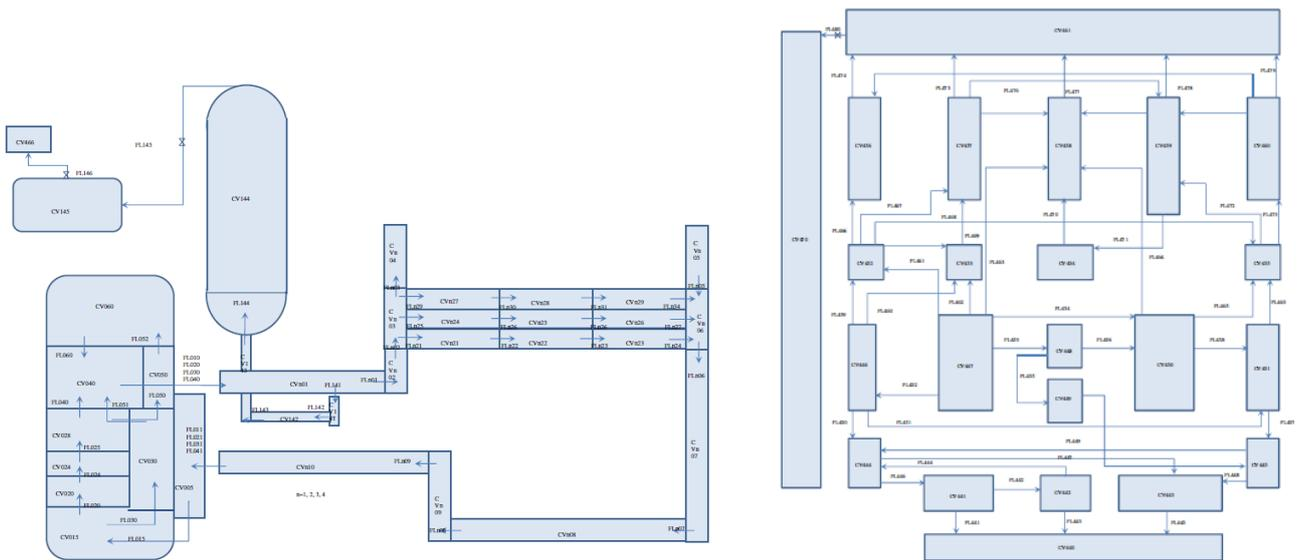
Figure 1. MELCOR containment nodalization scheme for VVER-1000/V320.
