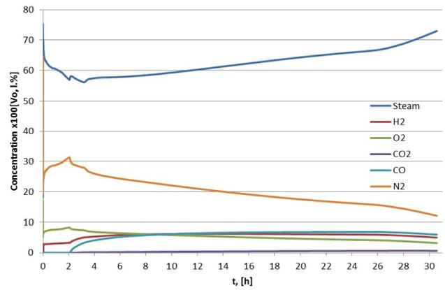
Figure 5. Volumetric concentration of the containment atmosphere components – dry case.
