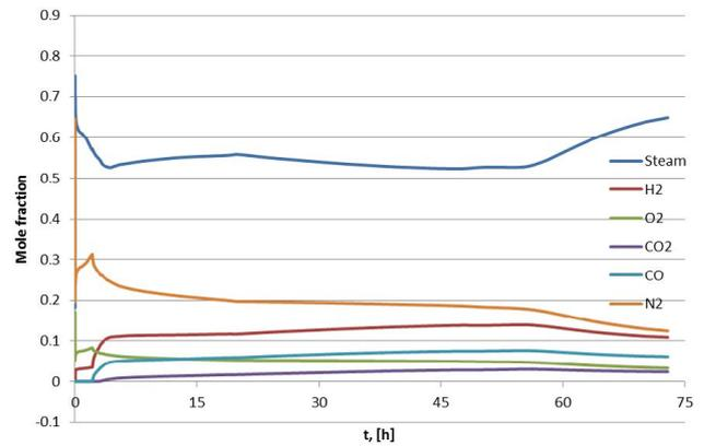
Figure 9. Concentration of the containment atmosphere components – two cavities case.
