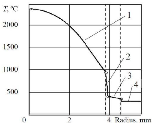
Figure 2. The radial temperature distribution in the fuel elements of the VVER.
