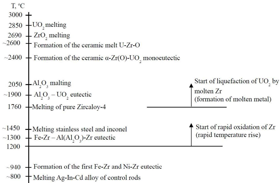
Figure 1. Typical phases of damage the reactor core with fuel  $UO_2$ .
