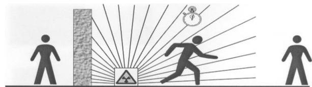
Figure 1. Shield, time, distance.
