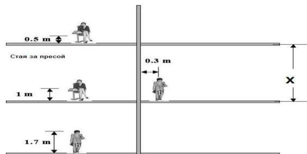
Figure 4. Distance for calculating rooms above and below PET facility.
