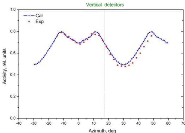
Figure 3. Example of calculated and experimental results for Fe detectors activity (in relative values).
