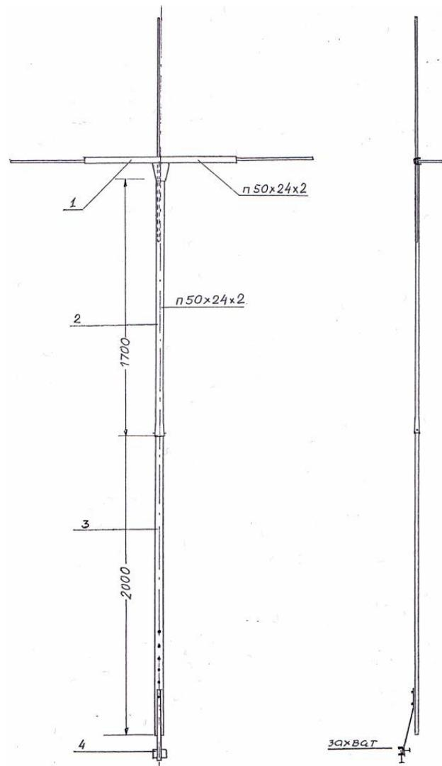
Figure 1. Supporting structure for the neutron activation detectors: 1 – cross-shaped holder for the activation detectors; 2 – upper part of the extender; 3 – lower part of the extender; 4 – bottom support.
