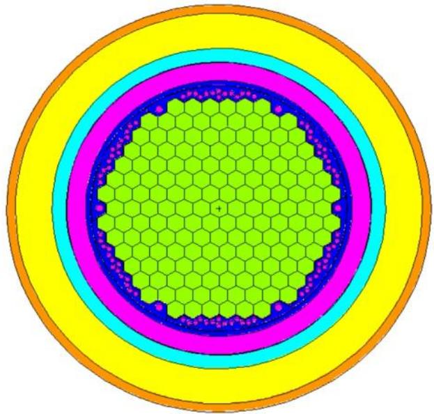
Figure 4. VVER-1000 MCNP model visualization in radial-azimuthal direction.
