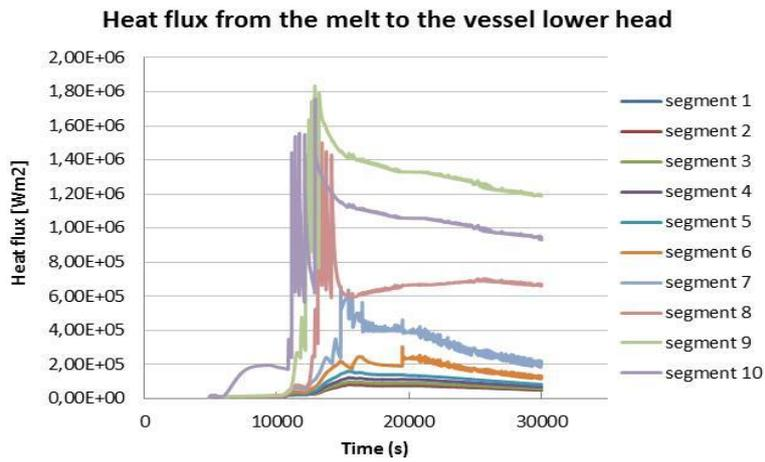
Figure 2. Internal heat flux distribution (ASTECv2.1.1.0 calculation).
