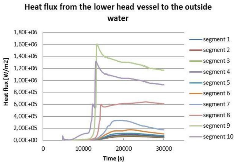
Figure 3. External heat flux distribution (ASTECv2.1.1.0 calculation).
