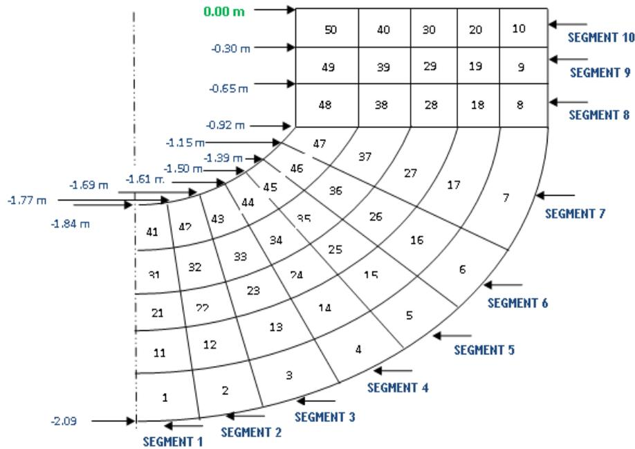
Figure 1. Segmentation of the vessel lower head for the ASTECv2.1.1.0 code modelling (elliptical section: segments 1-7, cylindrical section: segments 8-10).
