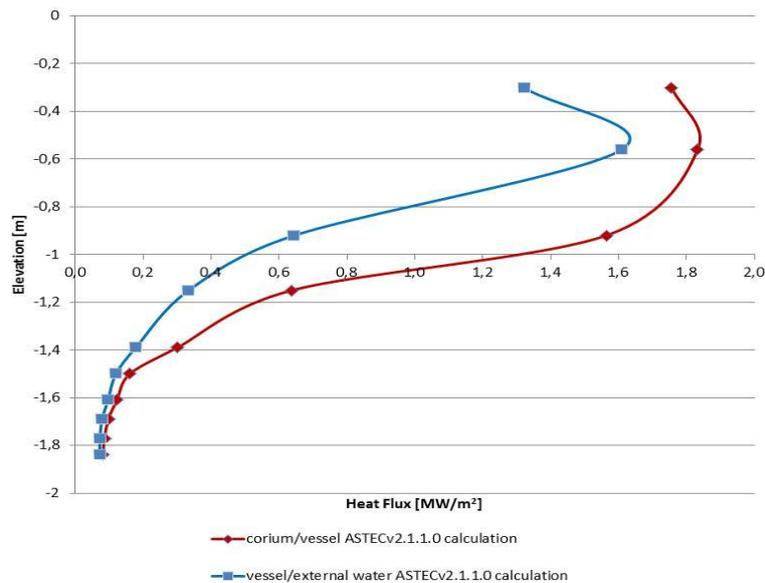
Figure 4. Bounding curves of maximal heat fluxes (ASTECv2.1.1.0 calculation).
