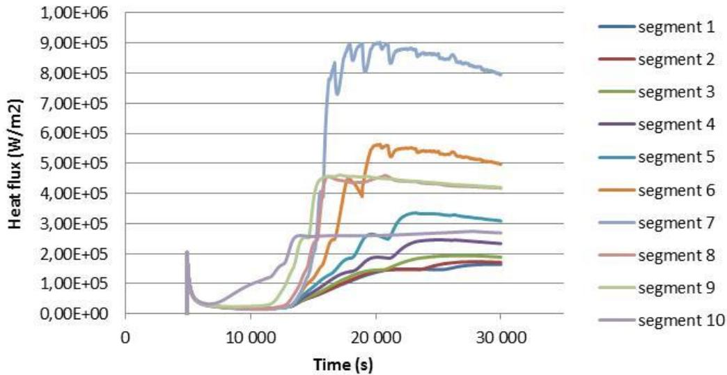
Figure 10. External heat flux distribution (ASTECv2.1.0.3 calculation).
