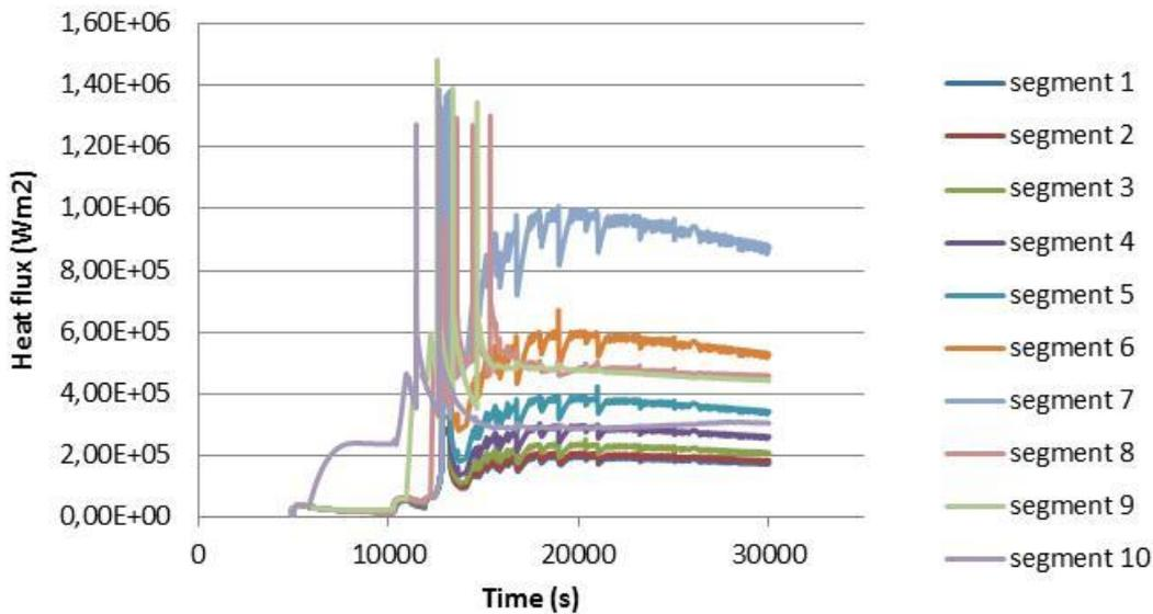
Figure 11. Internal heat flux distribution (ASTECv2.1.0.3 calculation).
