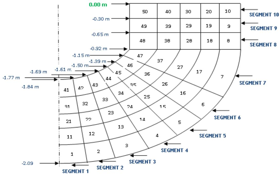
Figure 1. Segmentation of the vessel lower head for the ASTECv2.1.0.3 code modelling (elliptical section: segments 1-7, cylindrical section: segments 8-10).
