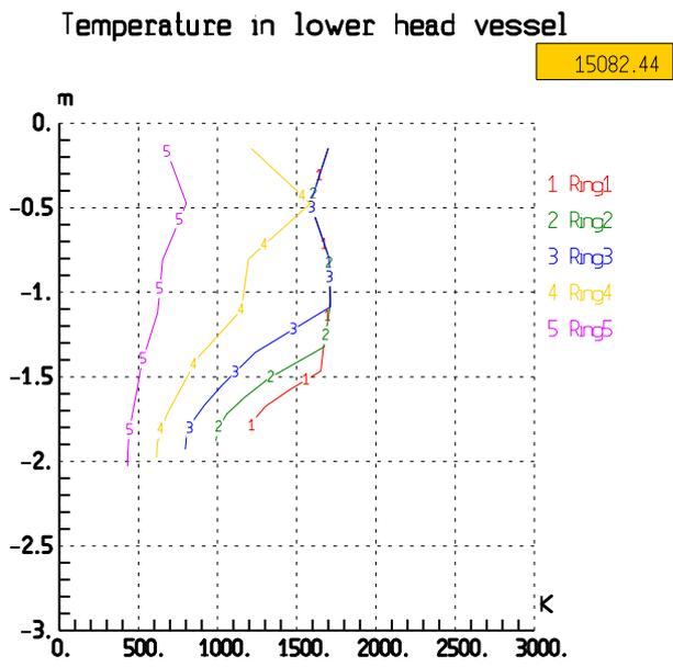
Figure 5. Rings temperature diagram at 15082 s.
