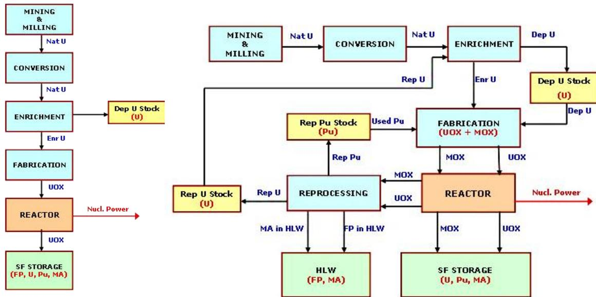
Figure 4. Fuel cycle diagrams, illustrating VISTA's material balance and flow calculation patterns – LWR once-through (left) and LWR closed cycle (right) [16].
