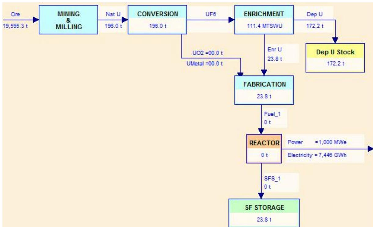
Figure 5. WWER once-through cycle material flows.
