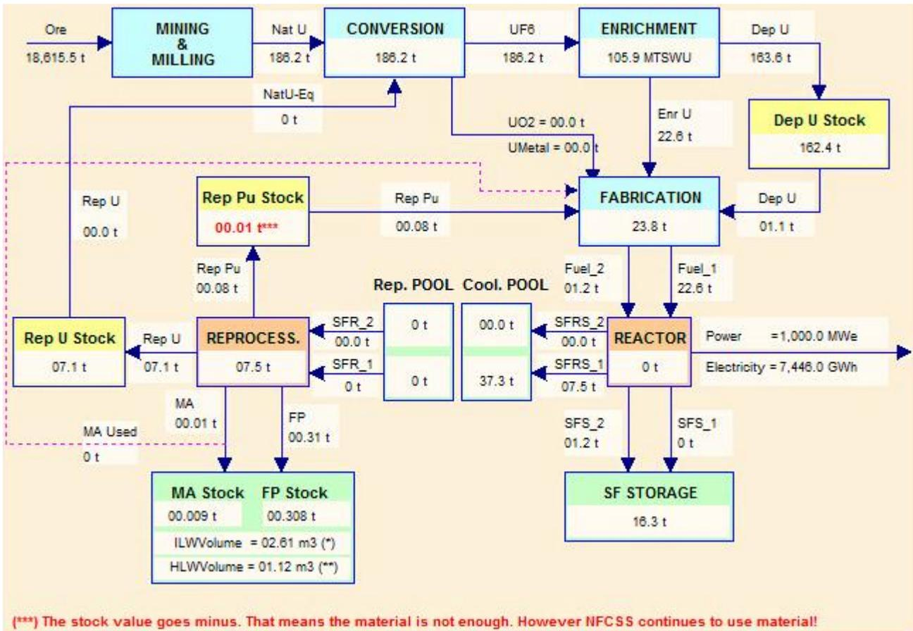
Figure 7. WWER partially closed fuel cycle material flows.
