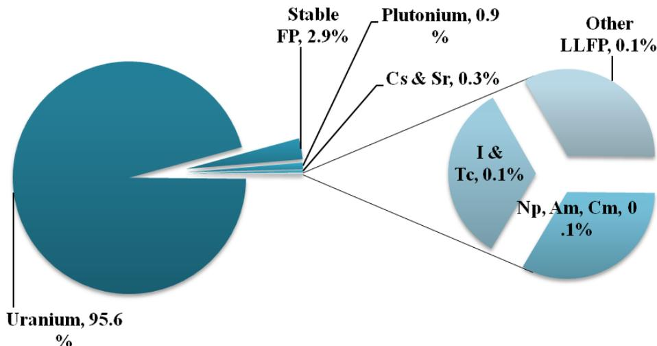
Figure 2. LWR SNF approximate composition, adapted from [9].
