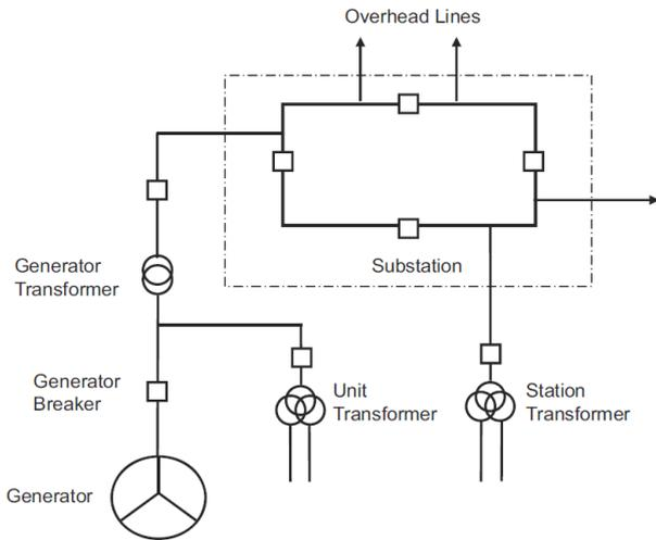
Figure 2. NPP connection to a single substation.
