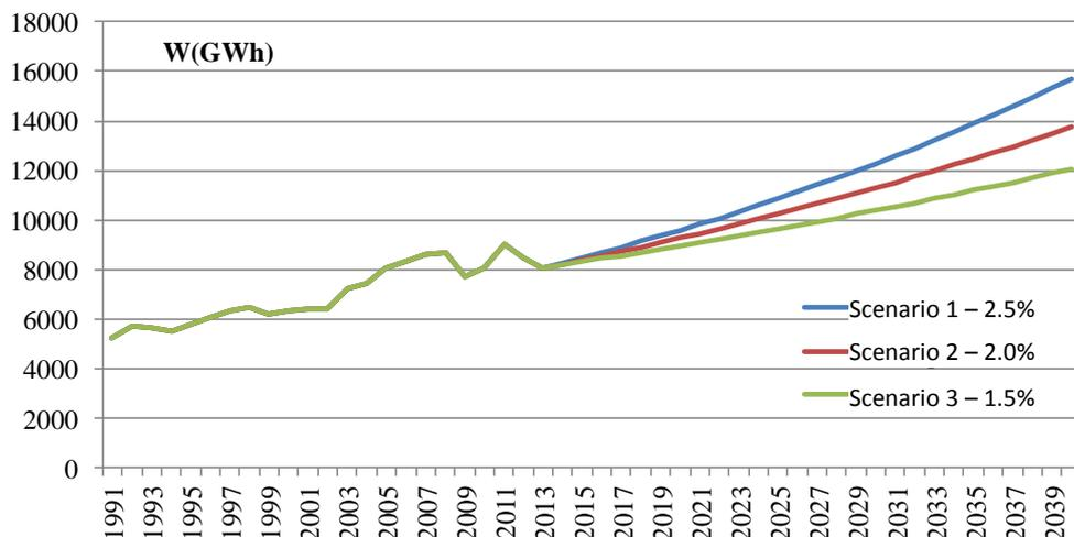
Figure 3. Forecast of electricity demand in Macedonian power system till year 2040.
