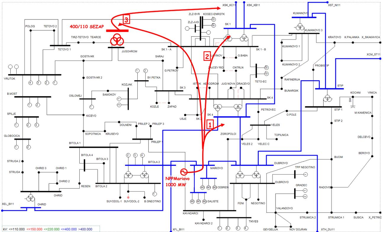
Figure 4. Long-term vision for development of Macedonian transmission grid and NPP integration.
